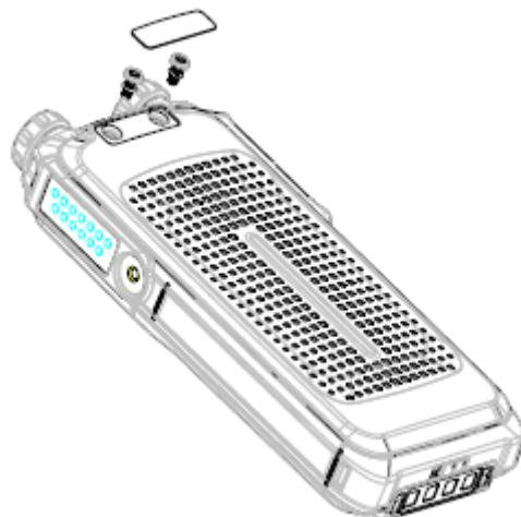
**Step 2** Remove the battery and unfasten the four screws.
