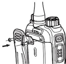
To remove the belt clip, loosen the screws.
