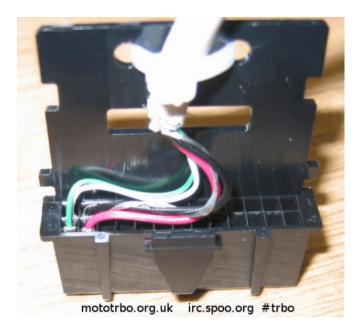
Note the bare (shield) wire is also crimped together with the ground wire.
