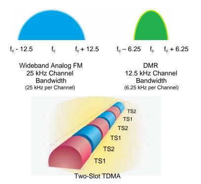
For the amateur, this means one repeater allows two separate channels at the same time. Currently most amateur DMR repeater system implementations utilize both channels for voice and some limited text messaging. Typically one channel (time slot) is used for wide-area and the second is local and regional Talk Groups.
