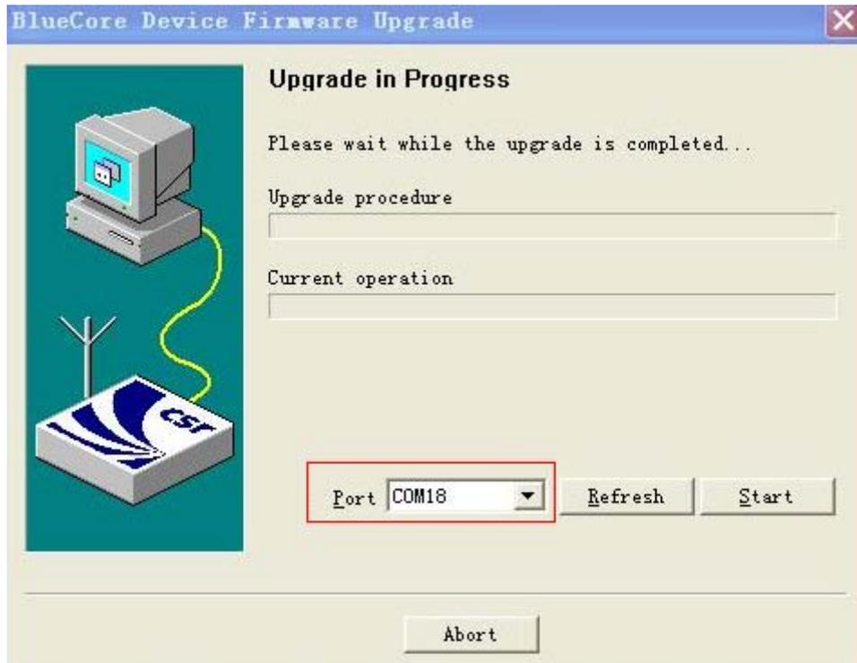
**Step 5** Select the appropriate COM port from the drop-down list of "Port". This port is used for connection between X1e/X1p and the computer.
