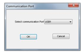
**Step 5** Select the corresponding USB port for the radio, e.g., USB 1, and click **OK**.
