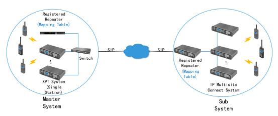
• One XPT system (master system) and two IP Multisite Connect systems (subsystems)
