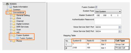
When **Call Type** is set to "Group Call", the groups in the master system and the subsystems must have the same **System ID**, so that they can communicate with each other.
