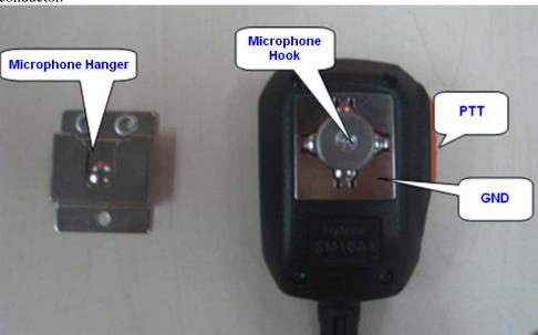
**Step 3** Hold the **PTT** on the palm microphone and power on the radio.
