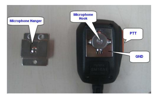
**Step 3** Hold **PTT** key on the palm microphone and power on the repeater.
