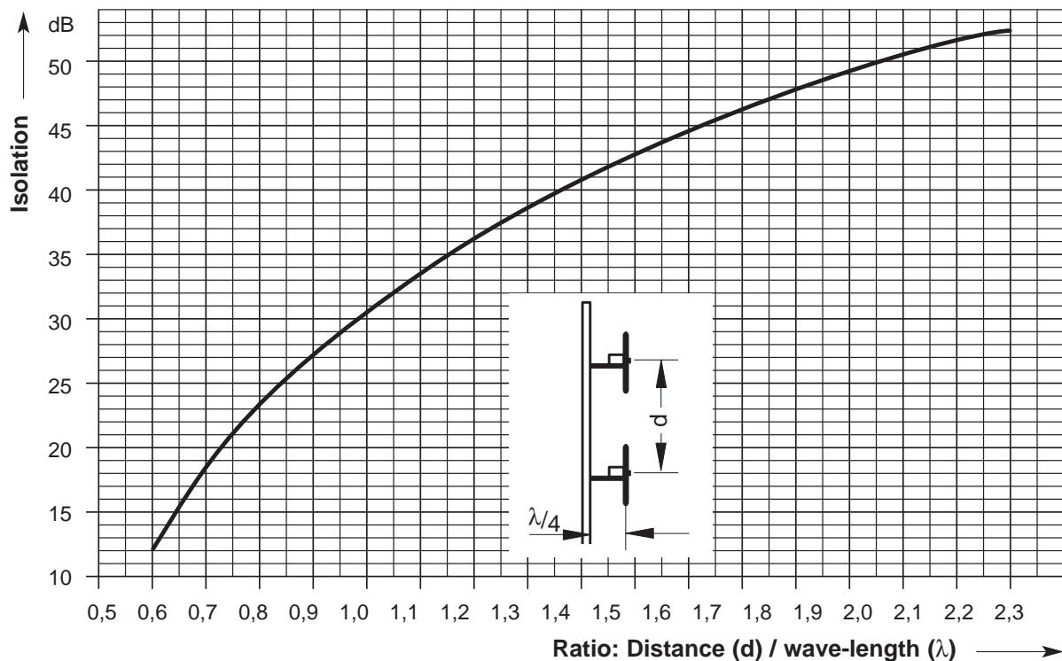
**Isolation** between two vertically polarized half-wave dipoles mounted laterally.
