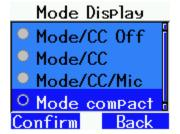
Select the option you want to use, Mode/CC will display operation mode and current ColorCode in the top status line. If you are using the Mic gain feature, you can optional display the current Mic gain setting in the top right corner of the advanced status line.
