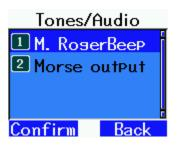
**M. Rogerbeep**: This lower the frequency of the sound that the radio makes when keying up. Only used if talk permit tone option is enabled in radio settings.
