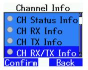
Channel info shows information of TS and TG below the selected channel and is being read from the codeplug settings of your radio. This provides more space for the channel name now, because most often this info has been added to the display name.
