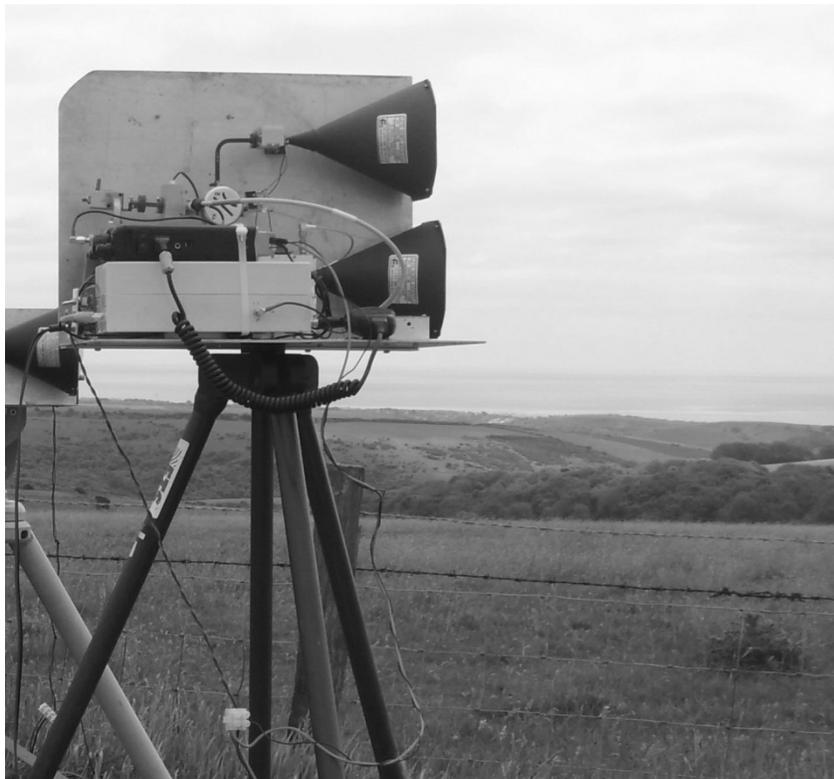
In Operation at Firle beacon with 10GHz transverter and FT817 fitted.
