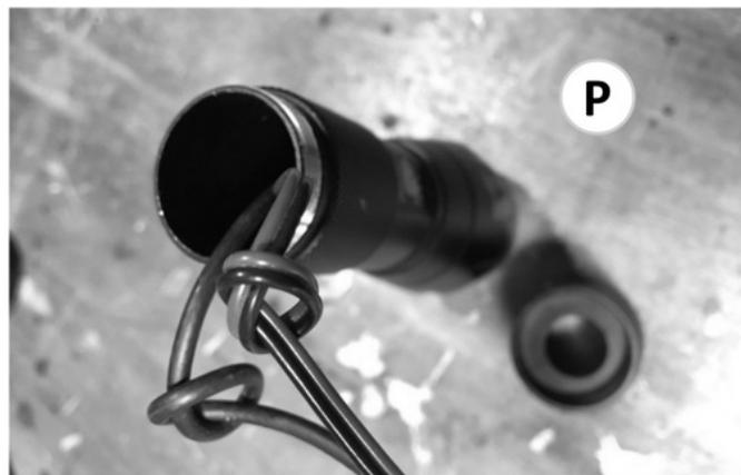
When you are happy that everything is working as expected it's time to reassemble your new lightwave transmitter. Start by press fitting the board back into the LED assembly (O).
