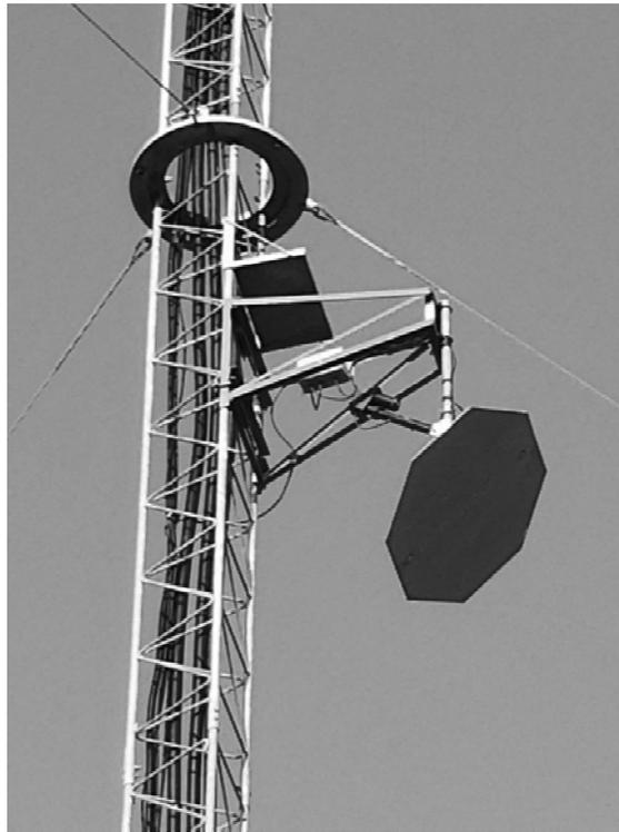
Figure 5. Flyswatter reflector with elevation/tilt control.
