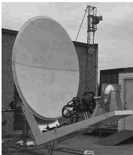
Figure 2. Tri-band SATCOM antenna
