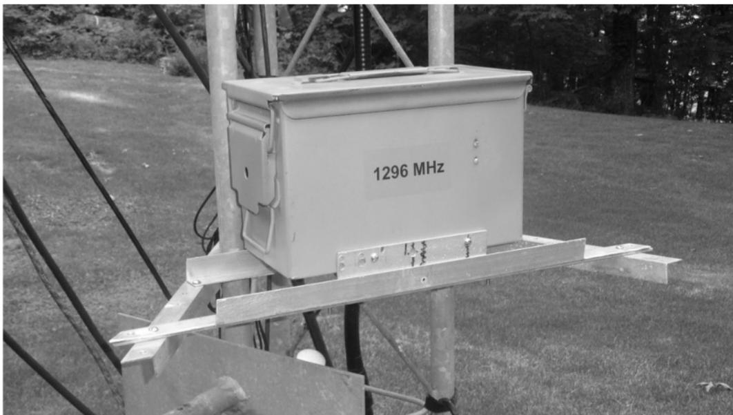
Figure 6 - RIG ATTACHED TO TOWER
