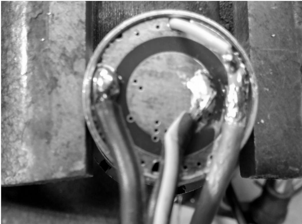
Figure 9 Power and Coaxial Driver Connections to PCB
