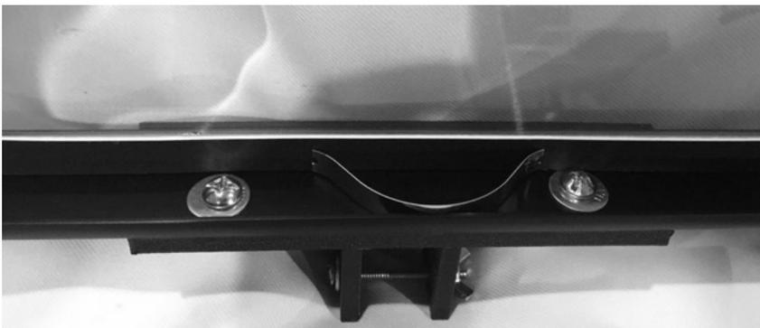
I use ¼ inch hardware to secure the frame to the mount, bolts, washers, and lock nuts. It creates a solid platform for holding the lens as well as making it easy to change the lens size.
