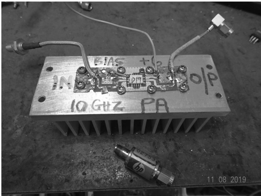
This Amplifier requires 2 Supply Rails... a Negative Bias Rail V<sub>gg</sub> (Green wire) of circa -0.20 Volts and +VDD Rail in the range +5 to +6 Volts maximum.
