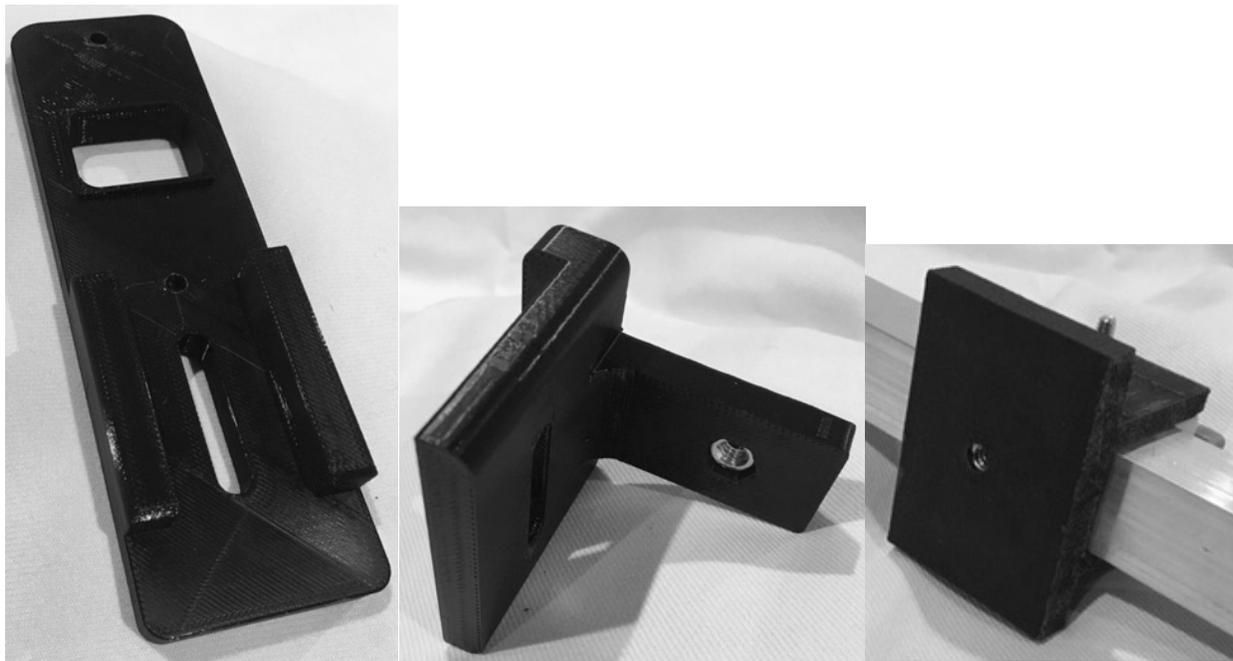
Individual parts for K0XL 3-axis mount; vertical slider, horizontal slider, base mount
