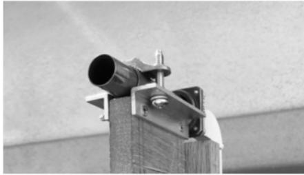
Horn Type: 3/4-in. copper    Aperture (mm): 20.6
