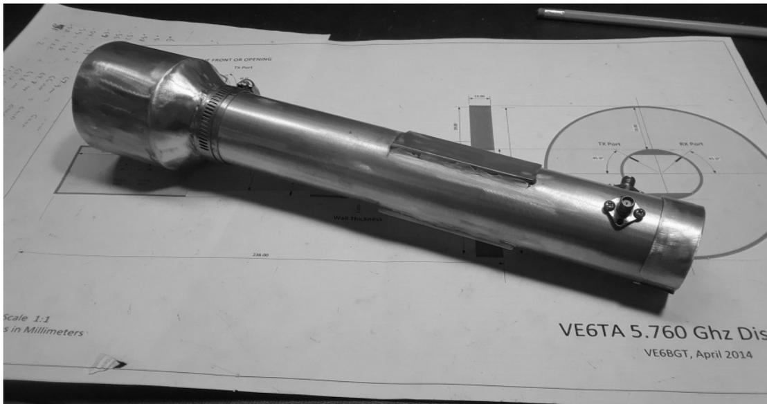
This picture shows the finished squeezed feed with the two plates soldered in and the new IMU launcher section. There is also an adjustable sliding back wall or plate to aid in tuning. I planned on using a SMA connector for the transmit probe only and usually a custom made receive connection made from a piece of .141 semi rigid coax to connect directly to the isolation relay, eliminating one connector for less line loss. I decided I would use the SMA connectors for both at first for the testing.
