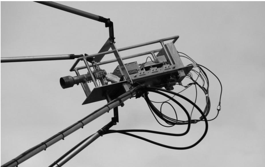
The new 6 CM feed assy. mounted on the 21 foot dish for final testing. Underneath is a feed position actuator to slide the assembly in and out for peaking on solar noise etc.
