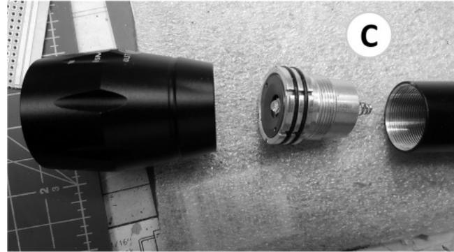
Remove the copper colored (inner ring) LED retaining ring. There is a clear spacer under the retaining ring, keep this as it protects the LED connections from shorting out. The LED and heat sink are now exposed. Unsolder the red (+) and blue (-) wires from the LED base (D). Clean off the LED assembly base and add new heat sink compound and add your new IR or red LED and solder it in place (E).
