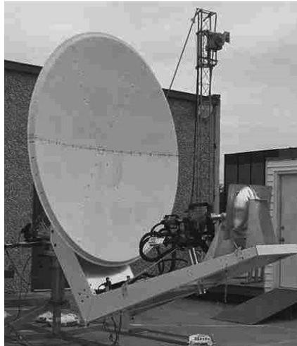
Figure 2. Tri-band SATCOM antenna
