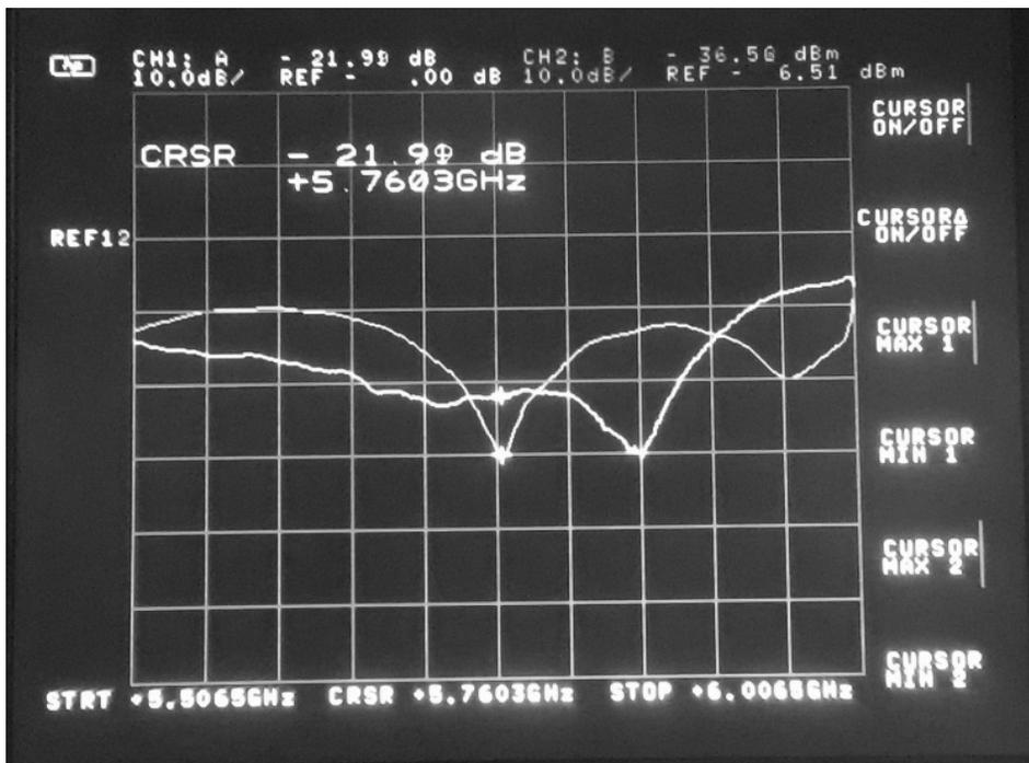
Twisting the IMU launcher section mounted on the end of the feed tube really shifted the RL dip of the TX probe off frequency. This showed me that the IMU section wasn't built concentric or true accurately enough.
