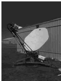
Transportable Tri-band SATCOM Antenna
