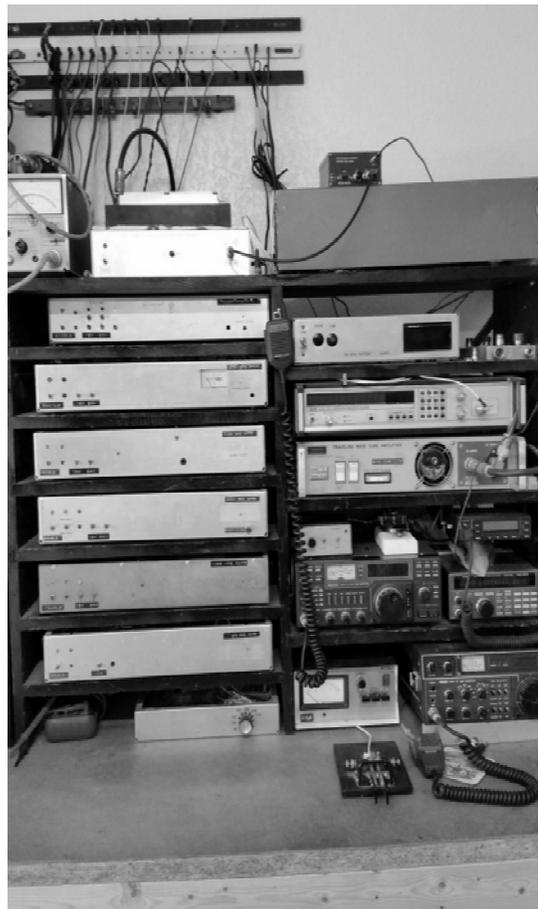
**Figure 2 AA5C Microwave Transverters**
