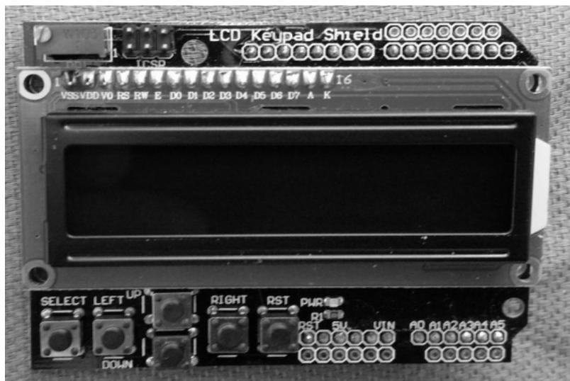
**Figure 5 2X16 LCD Display and Button Shield**
