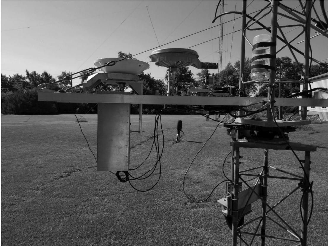
Figure 4. Equipment platform with both 77 GHz and 47 GHz transverters mounted
