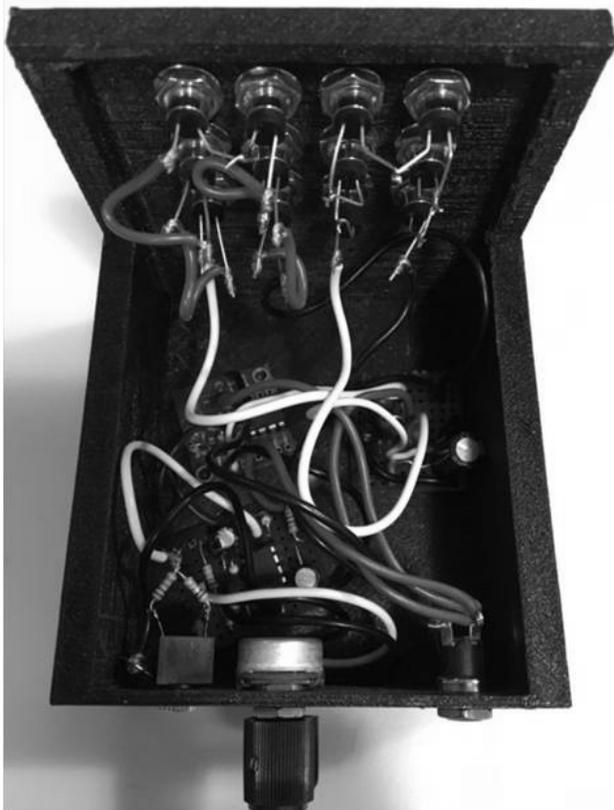
As you can see, it is not the prettiest of builds. Hidden under the wires are three small circuit boards, one for the microphone amplifier, one for the 555 timer modulator, and one for the LEDs driver module. It may be a bit ugly, but it works!
