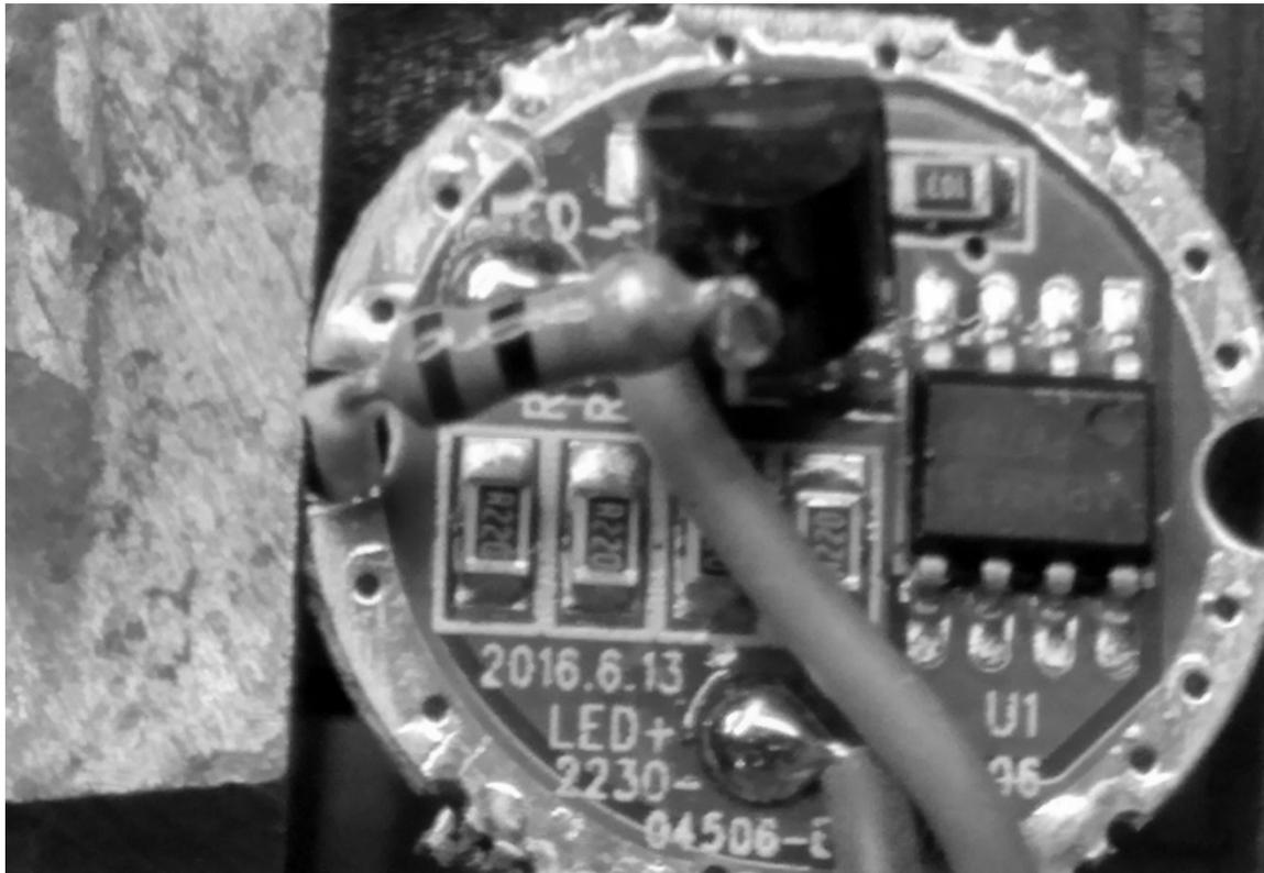
**Figure 6 2N2222 & 10 k Resistor Added**
