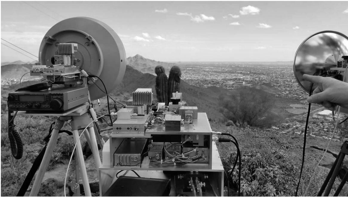
**Figure 12 N0IO & W7QQ 24, 47 & 78 GHz Setup on Shaw Butte**
