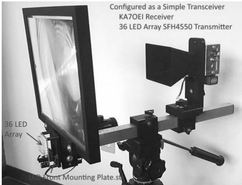
Rob designed 3D parts for mounting the 36 LED array on his receiver set up to create a simple optical transceiver.
