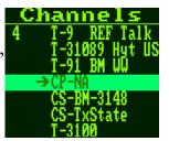
the top of the radio to a desired position in a zone, you can assign a channel to it by selecting 'Add to Zone'. Another option is 'Copy to Zone' which does the same thing, except it make a copy of the channel and applies the copy instead. This lets you change the settings without it affecting other zones you may have the channel assigned to. Don't forget to hit save after making any changes to
