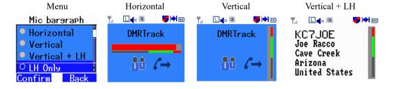
Creates a bar graph showing microphone activity on screen while transmitting. Try to keep the bar in the green area for optimal audio quality. User can choose from either a horizontal or a vertical bar. If using the vertical orientation + LH the screen will display the station information for the last station that transmitted before you keyed up. Very useful to remember call signs during a QSO because it is displayed in front of you while you are holding the PTT button.
