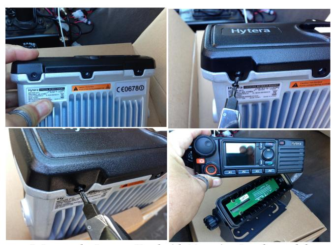
7. Locate the Remote Head with Mounting Bracket and the Hytera Control Head.
