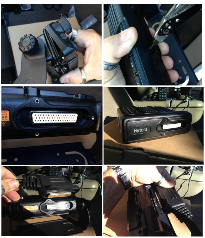
9. mate the Control Unit to the Remote Head mounting plate, verify it is seted, and install the 3 #6 Torx Screws. Install the Remote Head Cable to the Body, and to the Head unit.
