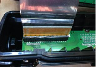
8. Line up the ribbon cable with the connector as before, gently push the ribbon cable into the connector, &verify it is seated.
