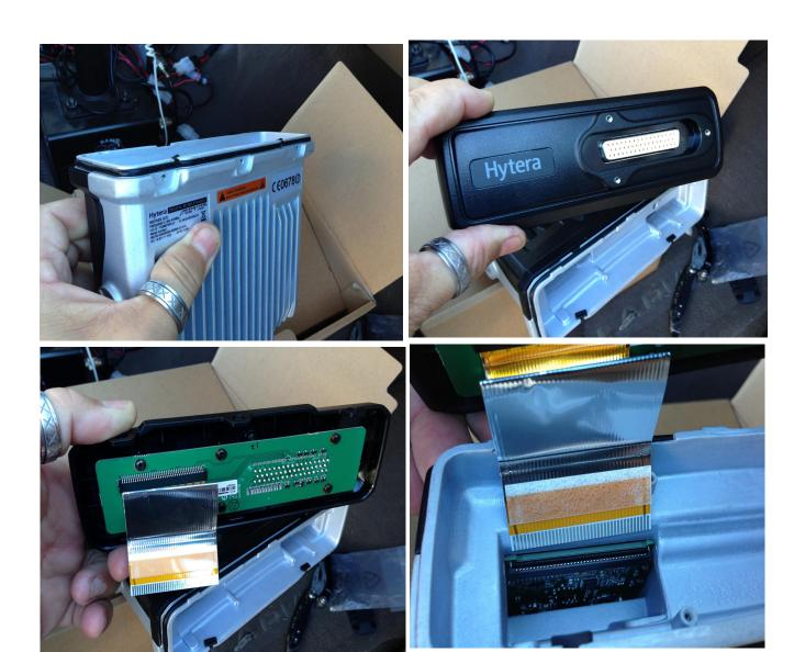
3. Orient the Control unit Remote Plate with the radio body.
