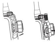
To remove accessories, loosen the screw.
